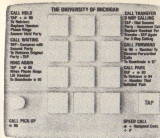
1.4 Plate Mounted Over the Dial of the Telephones at the University of Michigan. These inadequate instructions are all that most users see. (The button labeled “TAP” at the lower right is used to transfer or pick up calls—it is pressed whenever the instruction plate says “TAP.” The light on the lower left comes on whenever the telephone rings.)
